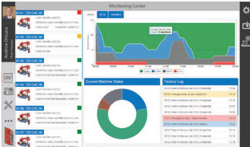
**BTM Connect automates the collection of the band saws' cutting data and analyzes operations to help staff on the plant floor measure and improve performance.**
