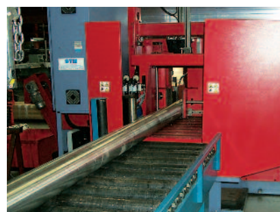
After ASA Alloys retrieves bar from storage, a loading cartridge places it onto a material handling conveyor in front of the 520 band saw.
