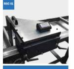
Mechanical length stop with sliding on iron pipe and manual lifting
