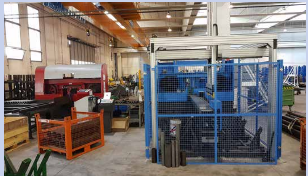
Special system for tubes and chromes cutting with internal cleaning. 12 m loading device
