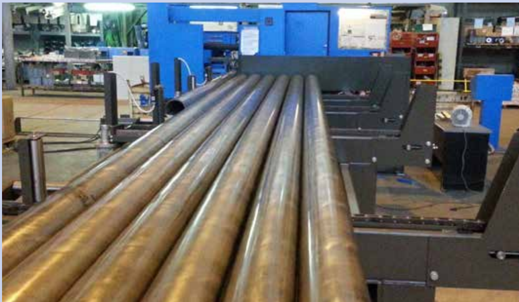
Loading system 6 m long
