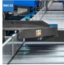
Powered length stop with sliding on iron pipe with encoder and hydraulic lifting
