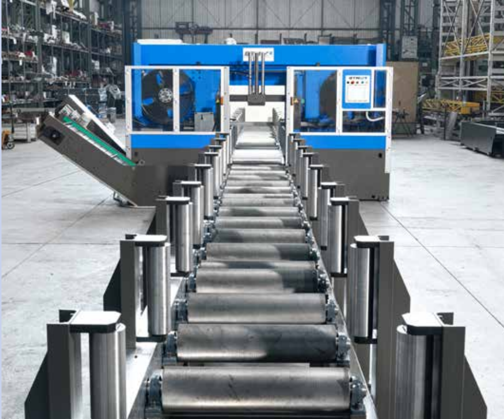
AT 740 SA F with infeed and outfeed roller track
