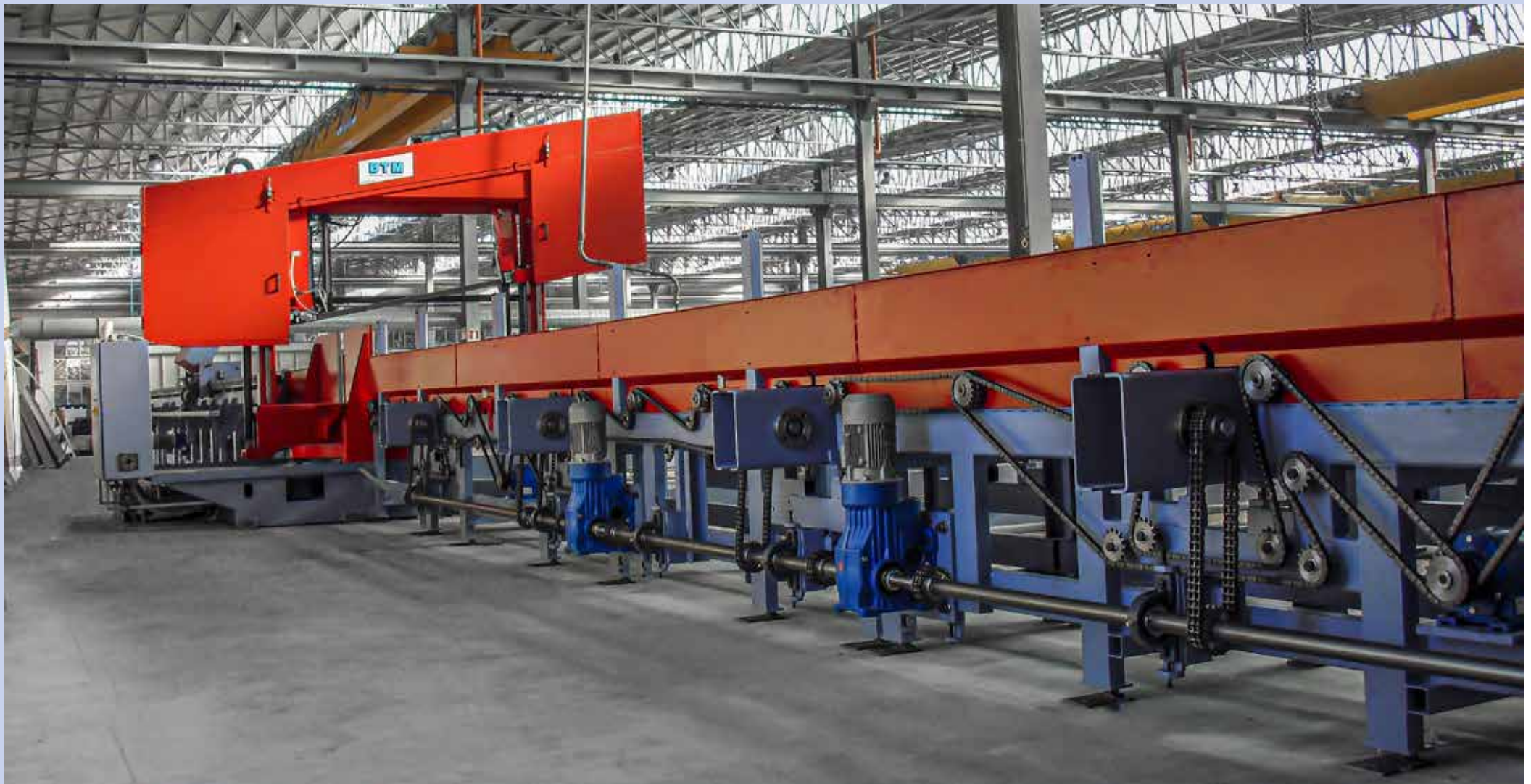
AT 12.7 SA DS with powered roller track, loading and unloading unit
